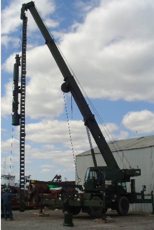
US Army custom pile driving system.
